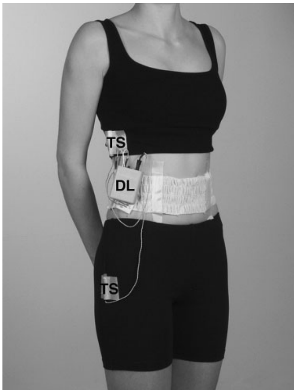
Figure 1 Photograph of a subject wearing the abdominal inductance plethysmography equipment. DL, the data logger; and TS, mercury tilt switches.
